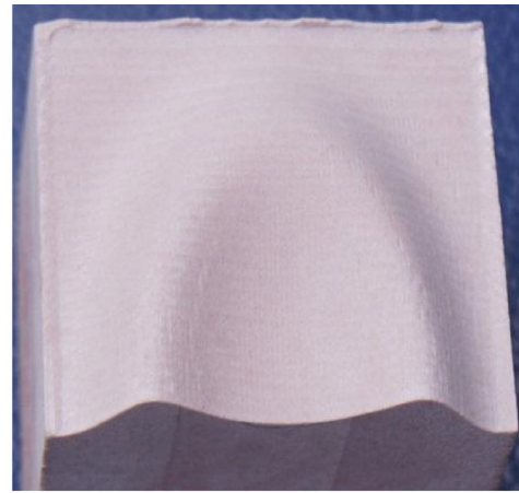
(b) Real machining, zigzag ISO, rough cut tool path length= 12034.0 mm, time = 2:01:03 hrs
