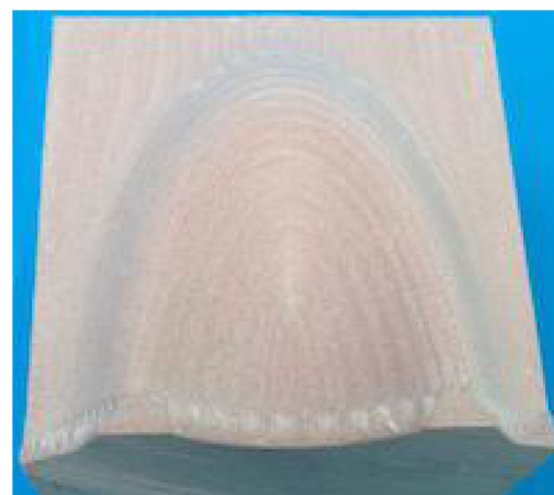
(f) Real machining VFAP R , rough cut, tool path length = 10075.0 mm ( advantage 16.3% ), time = 0:33:36 hrs ( advantage 72.2% )
